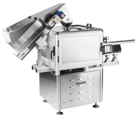
MULTIPLE LANE VIBRATORY FEEDER BELT PREFEEDER, SOUND PROTECTION STAINLESS STEEL STAND
