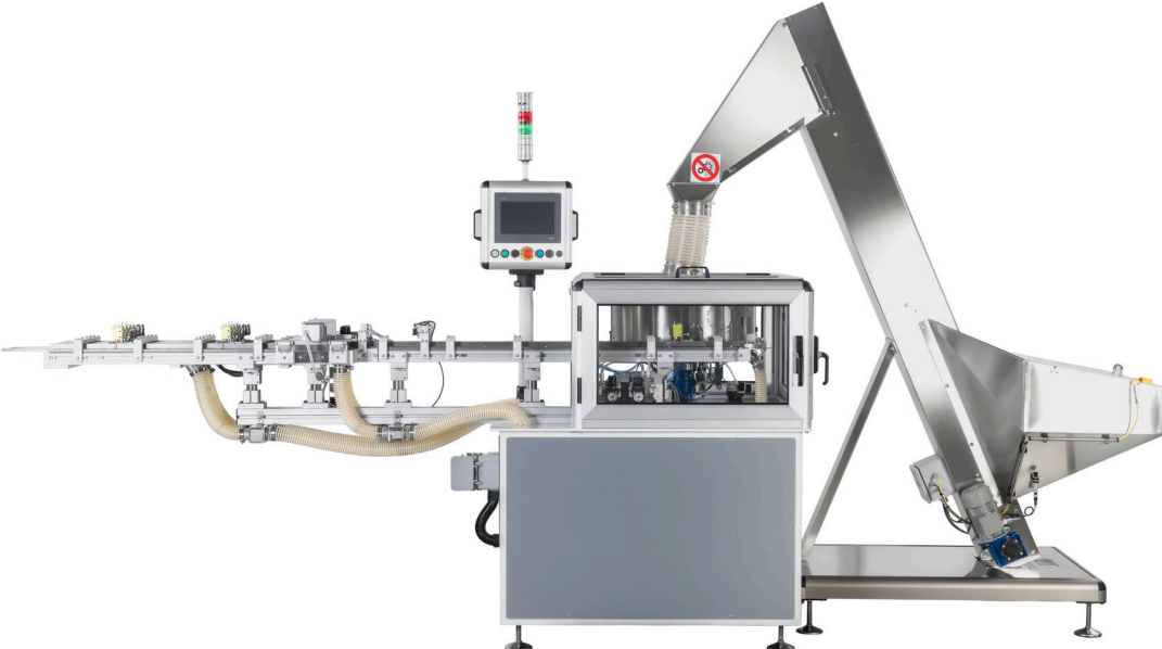
MULTIPLE LANE FEEDER WITH CENTRIFUGAL FEEDER STC FOR DISCS, CAPS, CAPSULES
